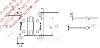
The basic footprint of the hinge is supported by previous fire testing on the H105 lift-off hinge (98 x 31 x 3 mm blade retained by 3No. fixings) and H1250 butt hinge (114 x 35/44 x 3.25 mm blade retained by 5No. fixings). The hinge also incorporates the concealed bearings already considered within this report.
