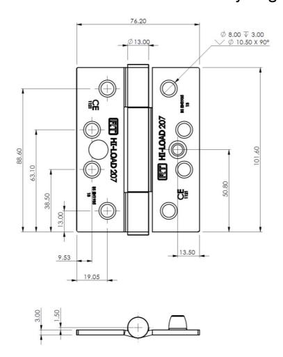
Security dog bolt version. Prevents removal of the door leaf if the hinge knuckle is attacked.
