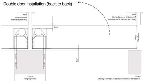
For a pair of conventional double doors an optional rebate to conceal line of sight can be used where no central mullion is desired.
