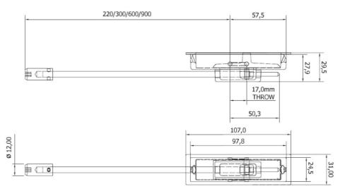
ANZ/R-220-FFD (220mm long) ANZ/R-300 -FFD (300mm long) ANZ/R-600-FFD (600mm long) ANZ/R-900-FFD (900mm long) "R" = radius R3mm
